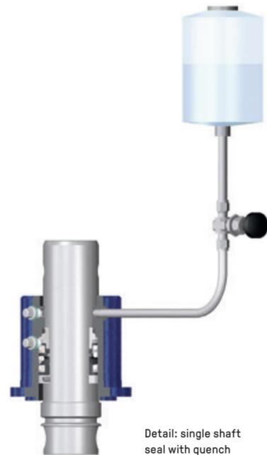
Detail: single shaft seal with quench
