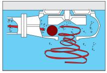
Impeller: virtually clog-free impeller with wide unobstructed passage in front.
