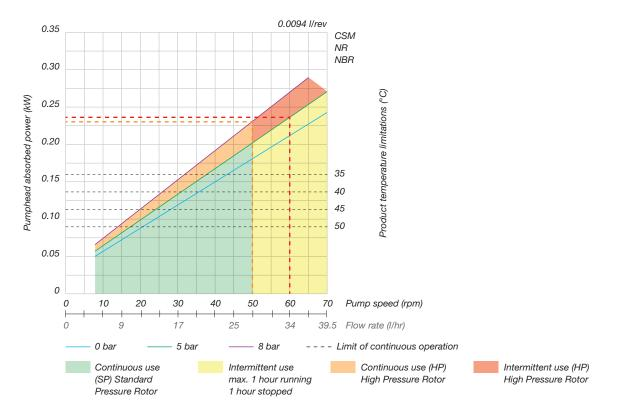
Any application below 15 Hz may require special review. Flows are typical and were measured with water at 20°C with no suction lift or discharge pressure. Actual flows will vary according to suction conditions, discharge pressure and normal component production tolerances.
