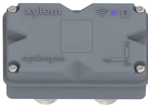
By periodically monitoring vibration, temperature and magnetic flux, optimize is able to identify potential problems with your equipment before they occur. Health information is collected, stored and analyzed in the optimize sensor before being wirelessly transmitted to your iOS or Android smart device via Bluetooth. The optimize mobile application provides an easy interface to understand the health of your assets, create maintenance reminders and generate detailed reports.
