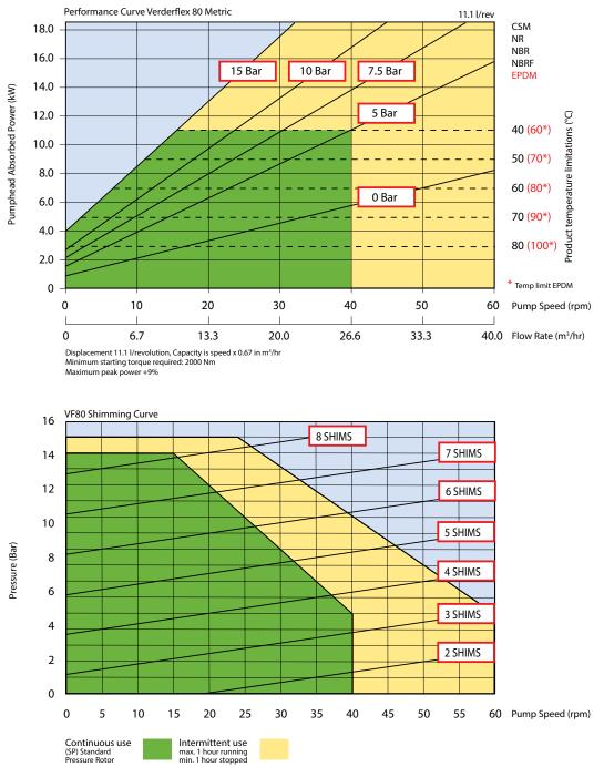
For product temperatures above  $65^\circ C$  and/or viscocity above 2000 mPas use one shim less than shown
