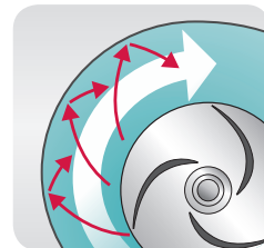
Standard impeller slams solids into the volute.
