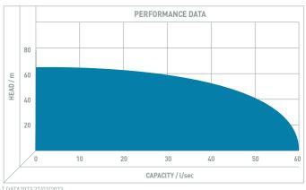
Due to the size range of the Jupiter tank, it is able to accommodate a wide range of pumping equipment giving a wide application range to a maximum of 60 l/s at 65m head.
