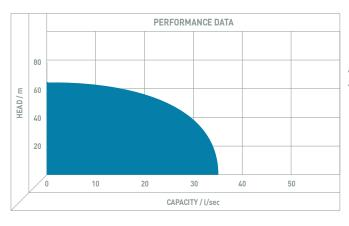
Due to the size range of the Saturn tank, it is able to accommodate a wide range of pumping equipment giving a wide application range to a maximum of 35 l/s at 65m head.
