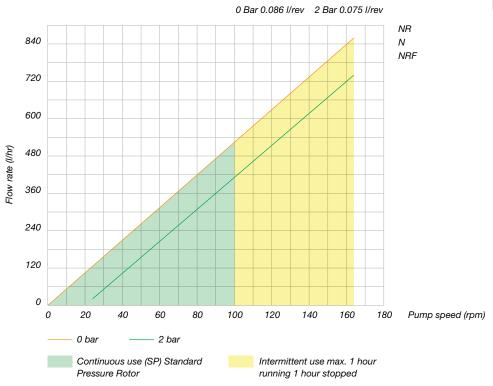
Flows are typical and were measured with water at 20°C with no suction lift or discharge pressure. Actual flows will vary according to suction conditions, discharge pressure and normal component production tolerances.
