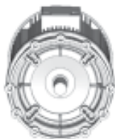
Fig. 8.3.1 A – Right location of the strainer on the motor flange
