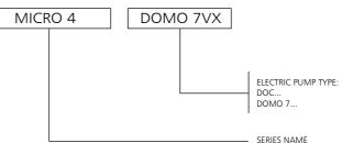
EXAMPLE : MICRO 4 DOMO 7VX Lifting station MICRO 4 series with DOMO 7VX submersible electric pump.
