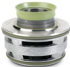
**PLUG-IN SEALS™** feature two independent mechanical seals (inner and outer) mounted in a single ready-to-install unit. No special service tools are required for installation and intelligent design protects sensitive sealing surfaces and springs from impurities. Selected variants feature our patented and leakage-preventing Active Seal technology.
